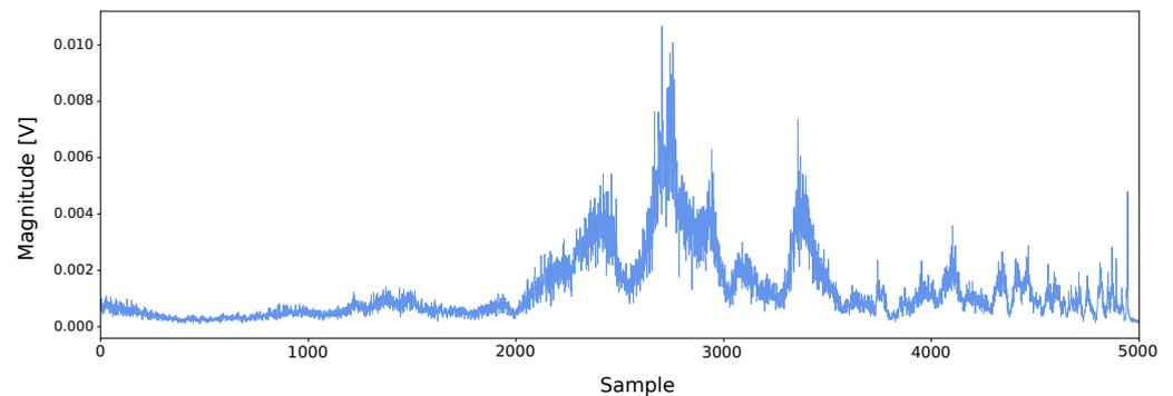
**Figure 13.** Results of the FFT from a vibration sensor placed in a cement ball mill.
