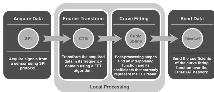
**Figure 11.** Data workflow within the expansion modules.
