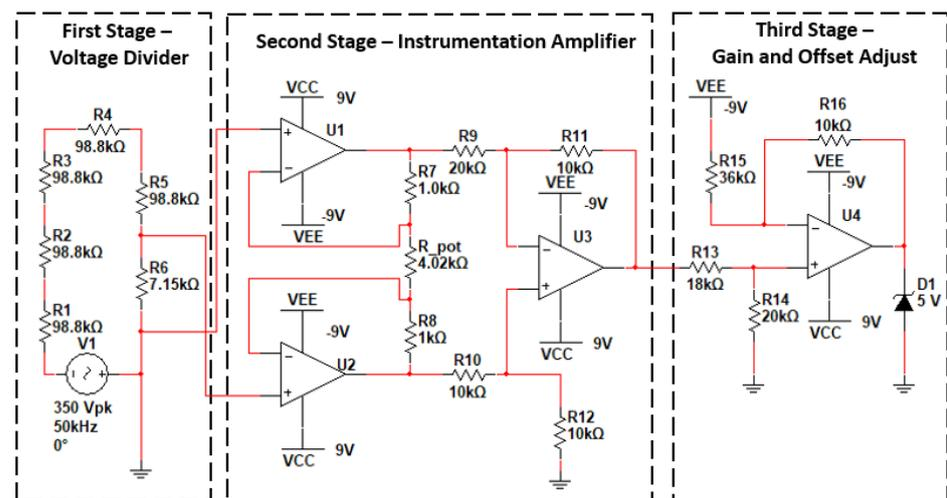
Figure 8. Conditioning circuit of the voltage signals.
