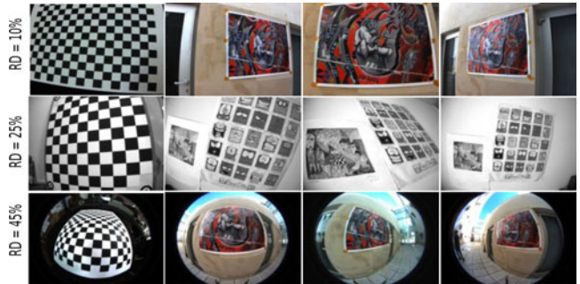
Fig. 4. Calibration grid and three images (out of 13) of each sequence used in the experiments described in Section V-A. The images were acquired with a camera with low lens distortion ( RD \approx 10\% ), a 4-mm minilens commonly used in flying robotics’ applications ( RD \approx 25\% ) [8], and a fish-eye lens with a wide FOV ( RD \approx 45\% ) [6], [7]. The resolution was 640 \times 480 for all cases.
