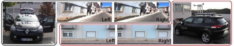
(b) Cameras mounted on a car and respective acquired stereo pair
