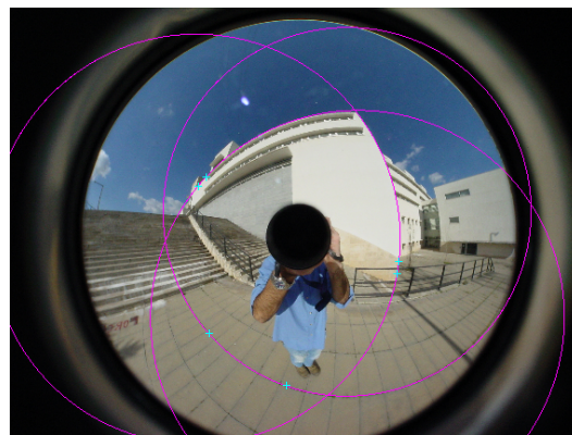
Figure 5: Estimating lines in a real image. The crosses are the points selected by hand
