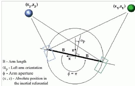
Figure 1. Vision System Configuration
