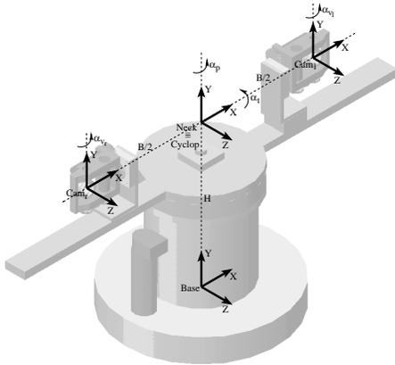
Figure 6. Binocular tracking configuration
