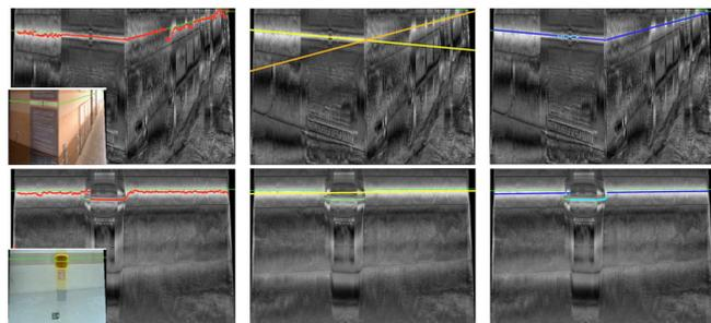
Fig. 7. 2 examples for the estimation of the profile cut location, green is the range data of the LRF. (a) estimated using Dynamic Programming (red), the correct location is only detected in textured regions or near strong edges; (b) lines (yellow and orange) detected using the hough transform, corresponding to the intersection of the virtual scan plane with planar scenes; and (c) MRF labeling decides between  $\mathcal{C}_{DP}$  (cyan) and  $\mathcal{C}_{s_i}$  (blue).
