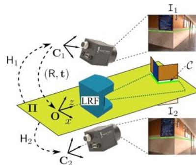
Fig. 1. Experimental setup. The top camera  $C_1$  (the reference view) points down, the bottom camera  $C_2$  points up, and the LRF is positioned between the cameras. The LRF recovers the profile cut  $\mathcal{C}$  that is the contour where the scan plane  $\Pi$  meets the scene structure.  $\mathcal{C}$  is projected in the two images  $I_1$  and  $I_2$  using the extrinsic calibration results.
