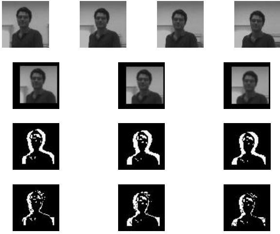
Figure 13: Image sequence acquired during monocular tracking. First row: Original images. Second row: Images after egomotion compensation. Third row: Set of image points with non zero velocity \dot{x} . Fourth row: Points used for target position estimation
