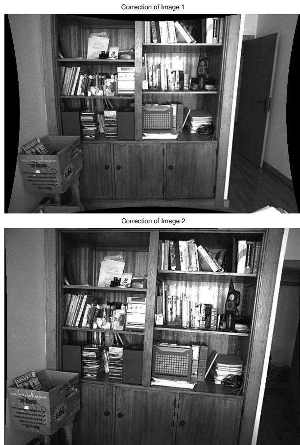
Figure 5. Correction of Radial Distortion. The distortion was estimated in 125.4 pixels for camera 1 and 22.9 pixels for camera 2
