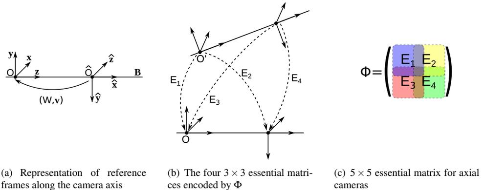
Figure 2: A new parameterization for axial cameras
