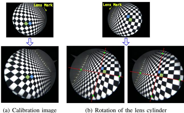
Fig. 3. Radial distortion correction under different environments and lens cylinder rotations. The distorted image (top row) is corrected independently of the lens cylinder rotation (bottom row). (a) The endoscope is calibrated for the lens position indicated in the top image. (b) Comparison between radial distortion correction without (left) and with(right) lens rotation compensation after a rotation of the lens.
