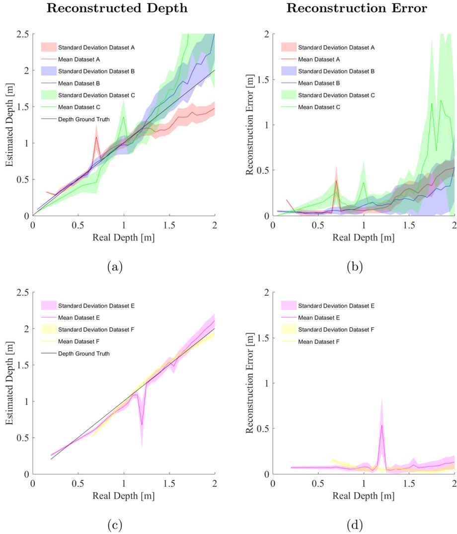
Figure 8: Reconstruction estimation accuracy with zoom step (**first row**) and with focus depth (**second row**). The **first column** depicts the reconstructed depth while the **second column** depicts the reconstruction error for the estimated points. The **first row** groups the datasets with focus depth at 0.05 m (Datasets A, B and C) and the **second row** groups the datasets with zoom step close to 336 (Datasets E and F).
