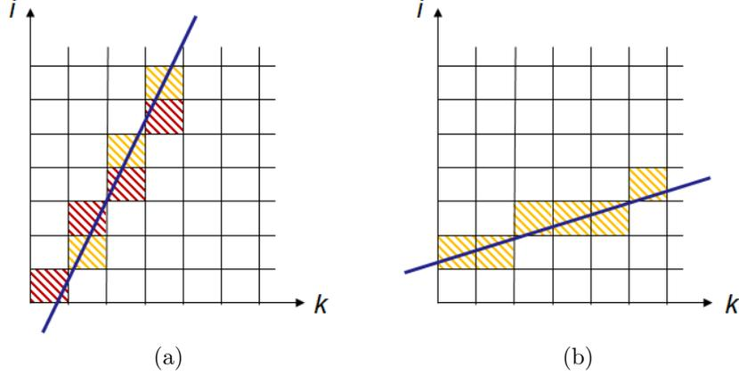
Figure 3: Rasterization method used to obtain the projections of a point  $\mathbf{m}$  for the  $(i, k)$  coordinates for different slopes of the projection line  $i = f^{-1}(k; \mathbf{m}, \mathbf{H})$ . The red pixels correspond to the projections skipped by assuming integer values for the microlenses  $k$ .
