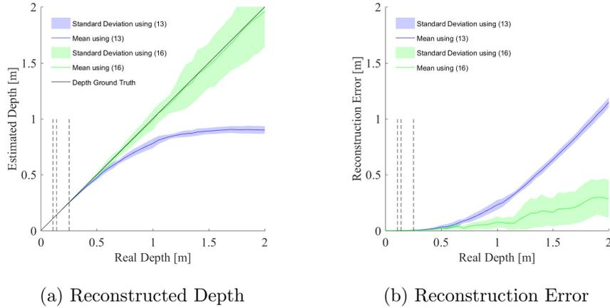
Figure 4: Results from reconstructing randomly generated points at depths ranging from 0.01 to 2.00 meters. The reconstructed depth is depicted in **(a)** while the reconstruction error using the  $(x, y, z)$  coordinates is depicted in **(b)**. (11) corresponds to the point reconstruction and (11) corresponds to the point reconstruction from line parameters. The dashed vertical lines, from left to right, mark the  $-2$ ,  $-1$  and  $0$  pixel disparities.
