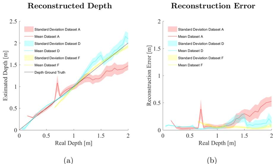
Figure 9: Reconstruction estimation accuracy with zoom step and focus depth. The **first column** depicts the reconstructed depth while the **second column** depicts the reconstruction error for the estimated points obtained for datasets with different zoom and focus settings.
