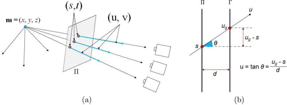
Figure 2: **(a)** Two plane parameterization for rays starting from a point  $\mathbf{m}$  using a point and a direction. Each of these rays correspond to different views of a point, i.e., they are samples of the lightfield. **(b)** The intersection of a ray with the two planes  $(s, t)$  and  $(u_g, v_g)$  define a geometry that allows to determine the direction of the ray. The plane  $\Pi$  defines the position of the rays while the plane  $\Gamma$  defines the direction of the rays.
