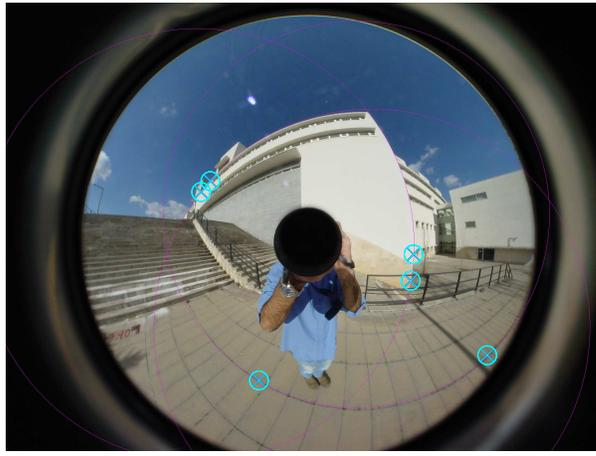
Fig. 12. Estimating the projection of lines in a calibrated paracatadioptric image using two points selected by hand.
