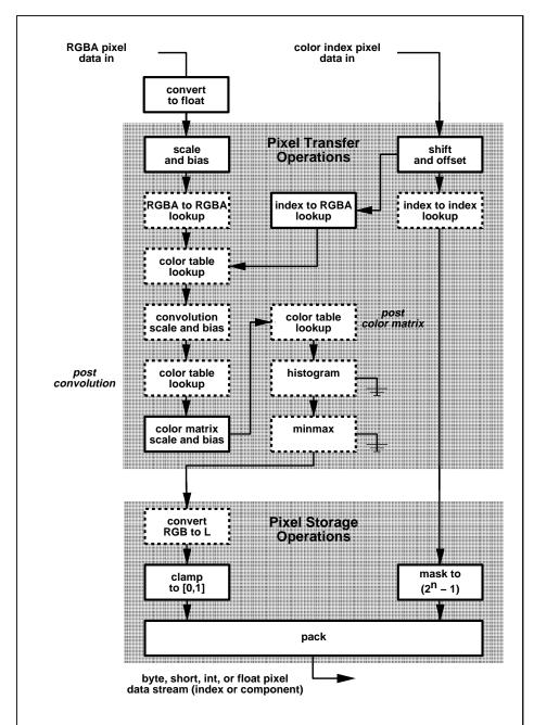
Figure 4.2. Operation of **ReadPixels**. Operations in dashed boxes may be enabled or disabled. RGBA and color index pixel paths are shown; depth and stencil pixel paths are not shown.
