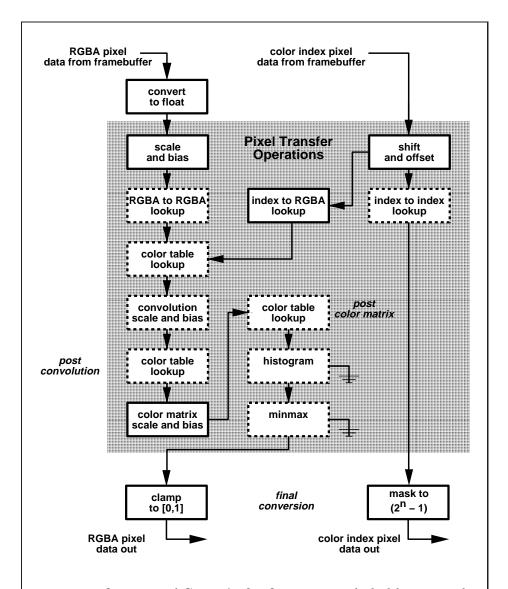
Figure 4.3. Operation of **CopyPixels**. Operations in dashed boxes may be enabled or disabled. Index-to-RGBA lookup is currently never performed. RGBA and color index pixel paths are shown; depth and stencil pixel paths are not shown.
