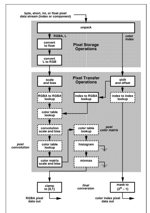
Figure 3.7. Operation of **DrawPixels**. Output is RGBA pixels if the GL is in RGBA mode, color index pixels otherwise. Operations in dashed boxes may be enabled or disabled. RGBA and color index pixel paths are shown; depth and stencil pixel paths are not shown.
