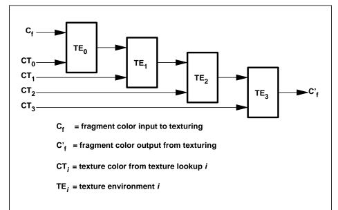
Figure F.3. Multitexture pipeline. Four texture units are shown; however, multitexturing may support a different number of units depending on the implementation. The input fragment color is successively combined with each texture according to the state of the corresponding texture environment, and the resulting fragment color passed as input to the next texture unit in the pipeline.
