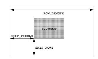
Figure 3.8. Selecting a subimage from an image. The indicated parameter names are prefixed by UNPACK\_for **DrawPixels** and by PACK\_for **ReadPixels**.
