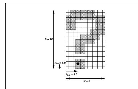
Figure 3.9. A bitmap and its associated parameters.  $x_{bi}$  and  $y_{bi}$  are not shown.
