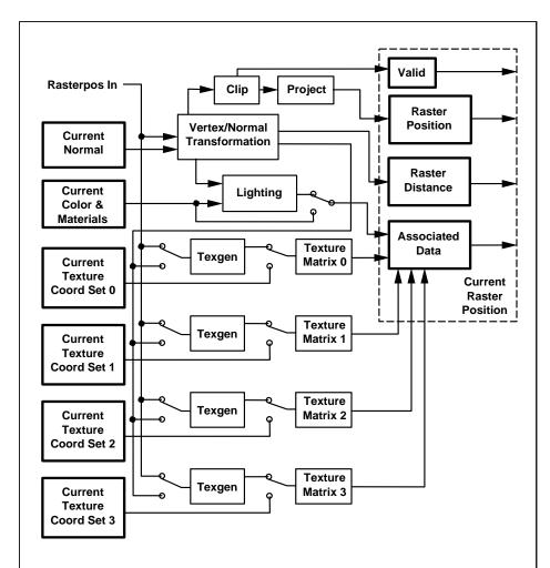
Figure F.2. The current raster position and how it is set. Four texture units are shown; however, multitexturing may support a different number of units depending on the implementation.
