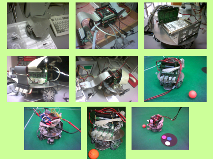
Fig.8 – Several stages of robot construction and assembly.
