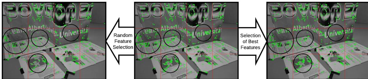
Figure 3.1: Matched features, using a random features selection (left), not limiting the number of features (middle) and selecting the best features (right).
