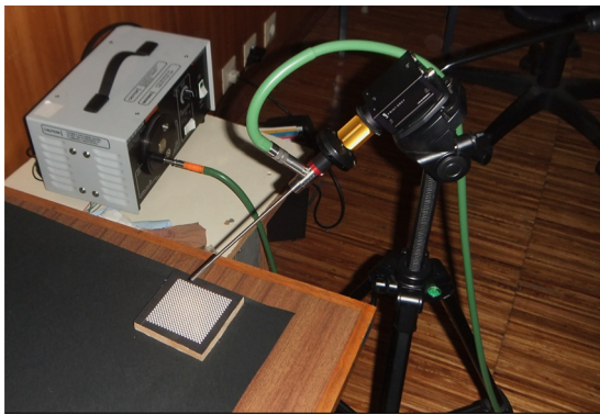
Fig. 1. Rigid oblique-viewing endoscope, used for image acquisition. The light source is connected to the boroscope through a fibre optic cable.
