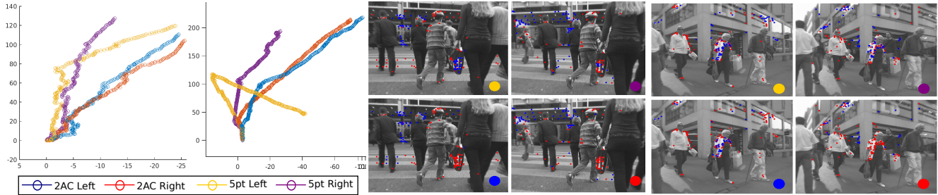
Figure 5: Experiment on the estimation of the essential matrix for a 220-image sequence (trajectories on the left) and a 600-image sequence (trajectories on the right) from the dataset presented in [5]. The estimation was performed for the left and right channels of the stereo pairs independently. The trajectories recovered for each channel, for the proposed 2-AC algorithm and the 5-point algorithm are identified with colors. For each sequence, an example showing the inlier (blue) and outlier (red) points is given. The stereo pair channel and used method are identified with a coloured circle.
